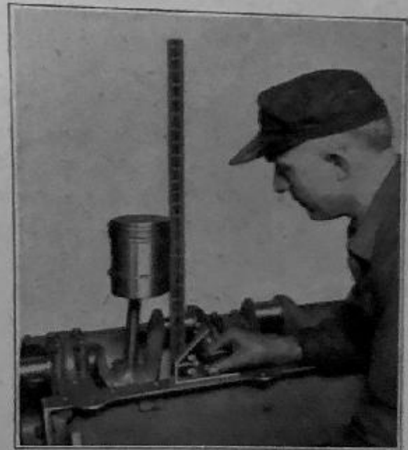
Lining up Pistons with Steel Square at End
