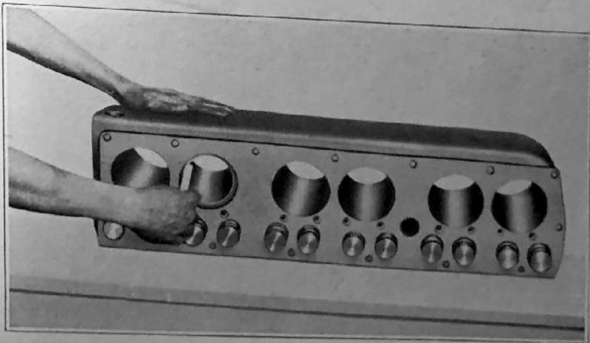
Checking Ring Gap in Cylinder with Feelers
