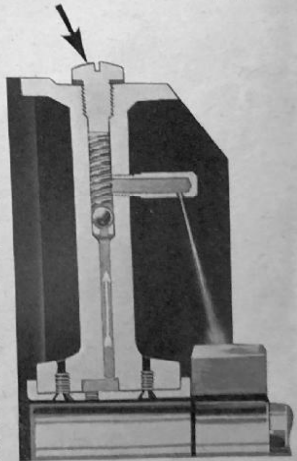
Oil Spray Nipple for Directing Oil on Timing Gears
