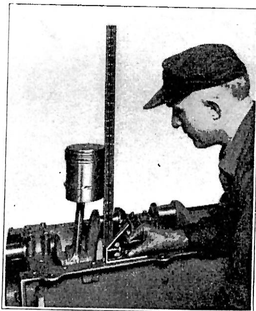
Lining up Pistons with Steel Square at End
